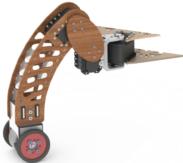
Figure 46: Diagram of a single leg of SigSent Robot demonstrating three jointed members.
