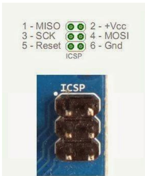
Fig. 37. ICSP Header and relevant pins
