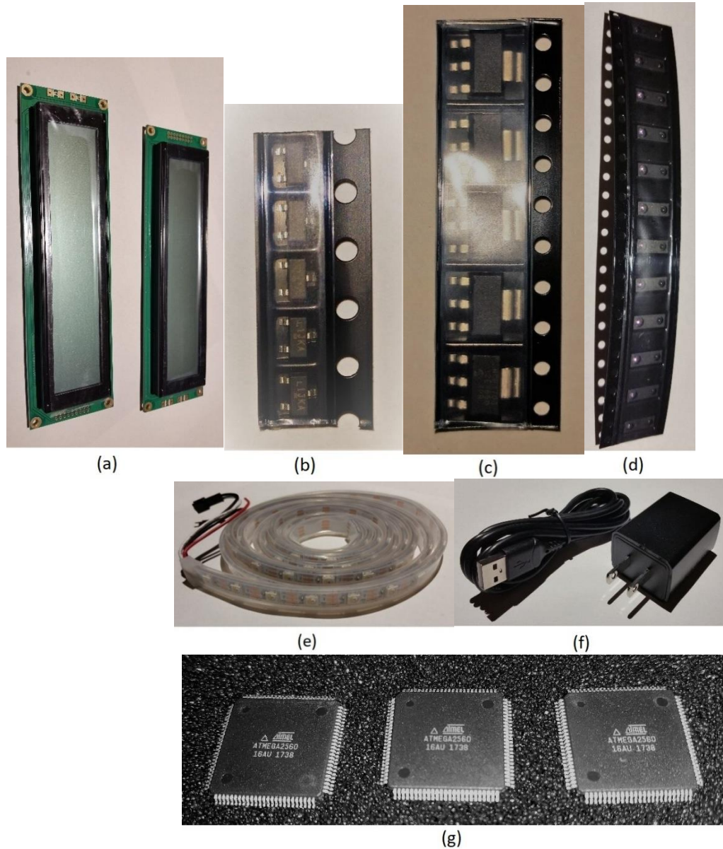
Fig. 39. The parts we ordered to build the prototype for our project, (a) the LCD screens, (b) the MOSFETS, (c) the voltage regulators, (d) the infrared sensors, (e) the LEDs, (f) the USB charger, and (g) the microcontroller processor chips.
