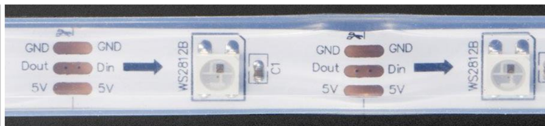
Fig. 19. A section of a strip LED with waterproof coating. The connections may be cut and soldered as needed.
