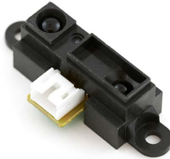
Fig. 37. The Sharp GP2Y0A41SK0F infrared proximity sensor. We changed to this sensor due the difficulty in getting the Vishay VCNL4200 to work.
