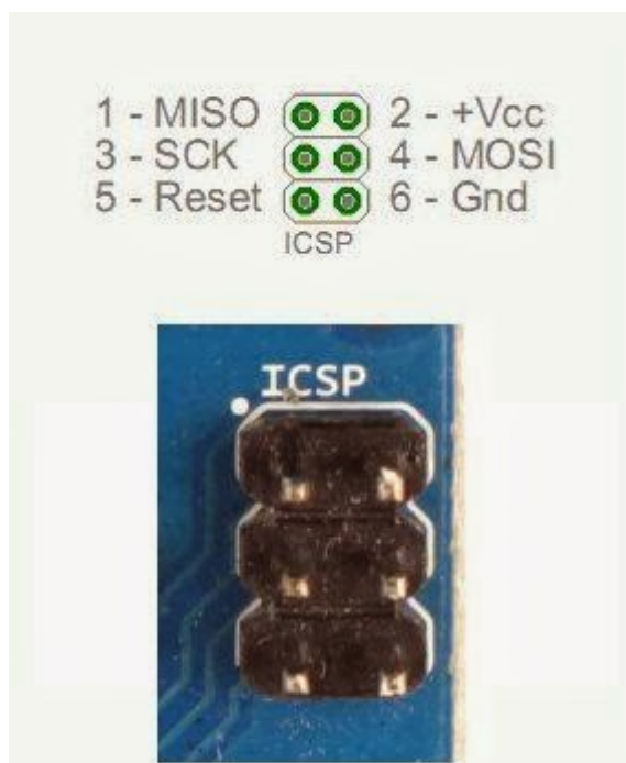
Fig. 43. ICSP Header and relevant pins
