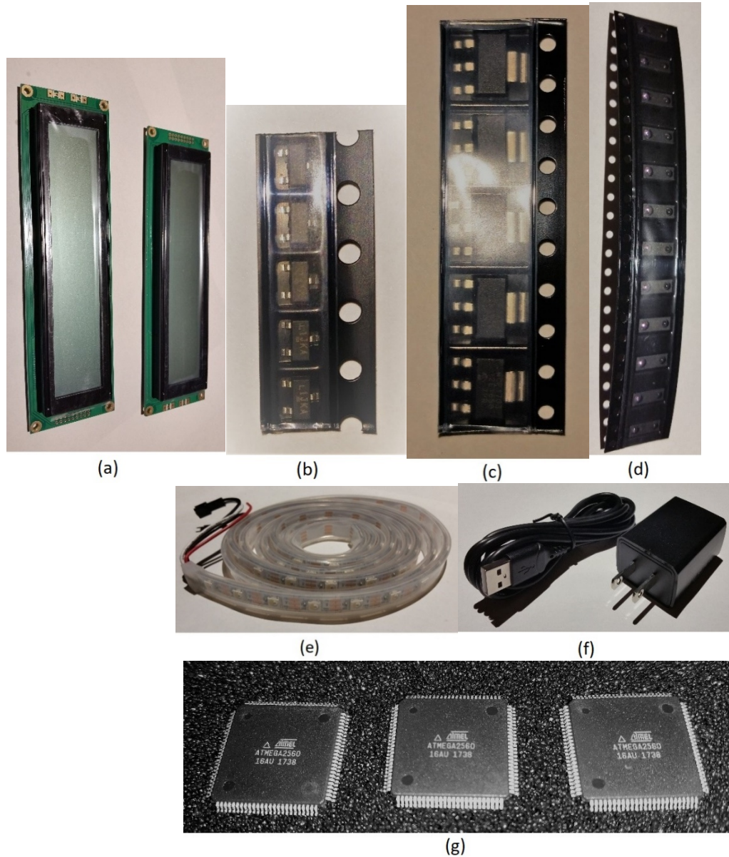
Fig. 45. The parts we ordered to build the prototype for our project, (a) the LCD screens, (b) the MOSFETS, (c) the voltage regulators, (d) the infrared sensors, (e) the LEDs, (f) the USB charger, and (g) the microcontroller processor chips.
