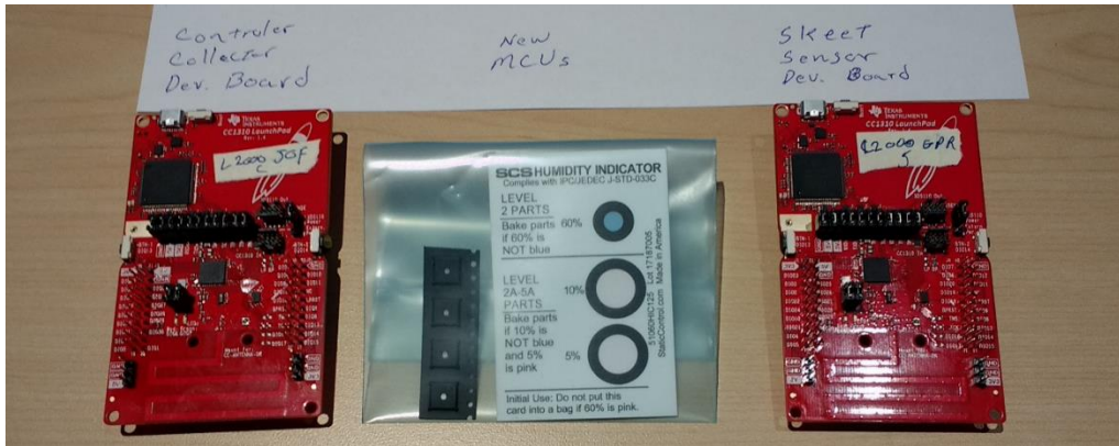
Figure 27 - Parts, MCU Components
