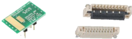
Figure 8 – Custom LCD PCB, Ribbon to Pin adapter
