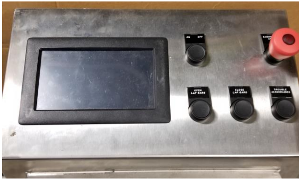
Fig. 2. The HMI, showing the touch screen, open lap bar, close lap bar, trouble acknowledge, and emergency stop buttons.
