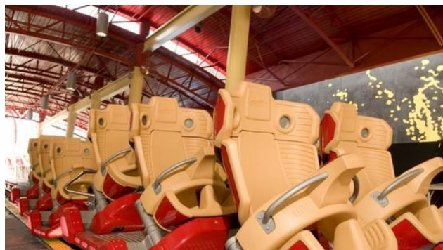
Fig. 1. The Hollywood Rip Ride Rockit ride vehicle and lap bars.
