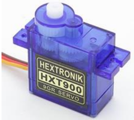
Figure 11: 9-Gram Servomotor [15, reprinted with permission from Hobbyking]
