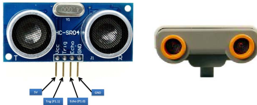
Figure 14 – Typical Distance Measurement Ultrasonic Sensors
