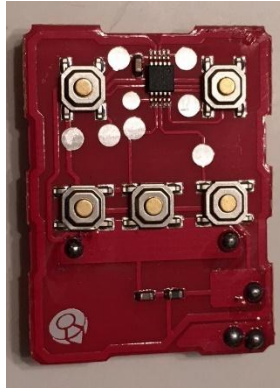
Figure 46: Image of internal PCB of key fob
