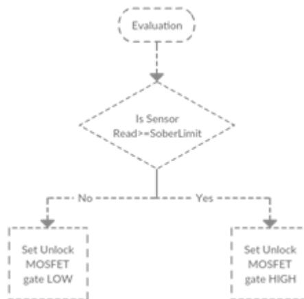
Figure 37: Evaluation process demonstrating the unlocking phase that allows the user to use the button
