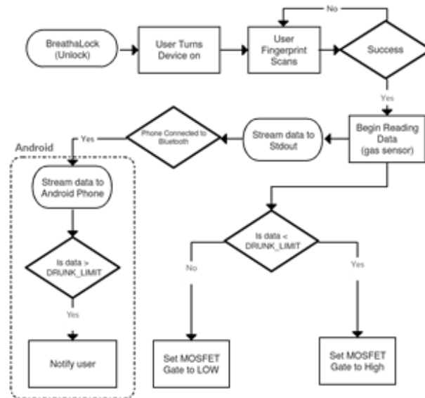
Figure 38: Software Flow Diagram including our android portion
