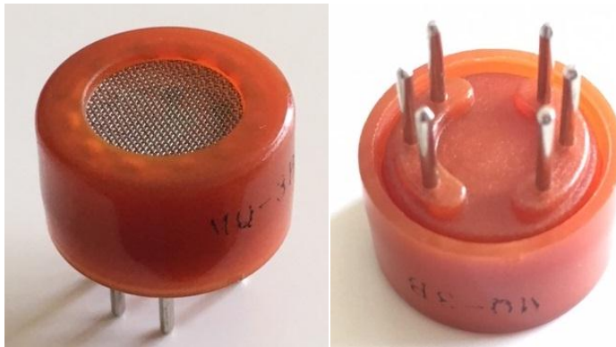
Figure 11: MQ-3 sensor external image and pin reference
