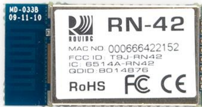
Figure 6: Example of Bluetooth unique 48-bit address.
