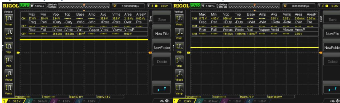
Figure 5-12 12-volt DC signal
