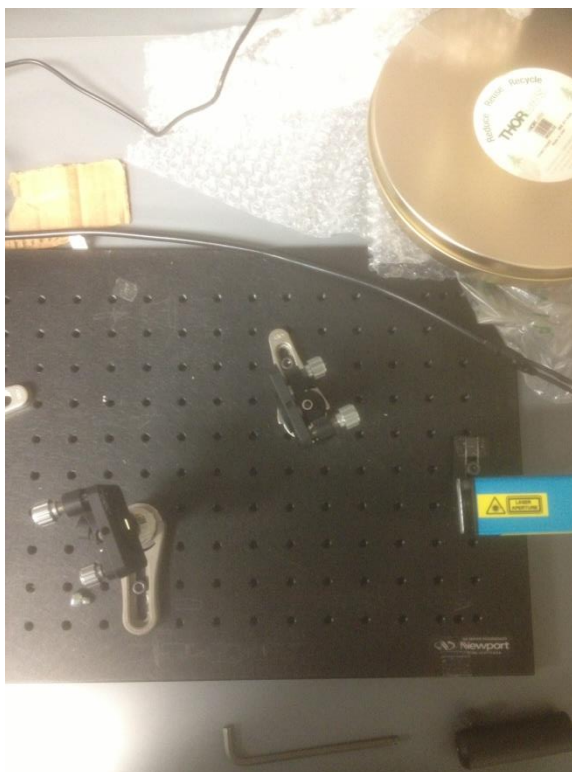
Figure 22: Optical setup with the 785 nm laser and the two RBG's
