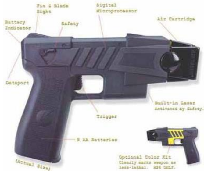
Figure 4: Layout of how a typical stun gun works
