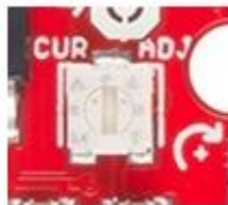
Figure 5.3.10 – The Potentiometer on the EasyDriver Board
