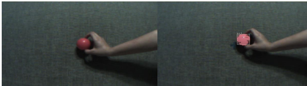
Figure 6.2a - Test Case 1 images. Captured in PixyMon. On the left, object to be tracked is presented to Pixy Camera. On the right, the Pixy Camera registers the object's color signature and begins tracking the object after being prompted by a command from PixyMon.
