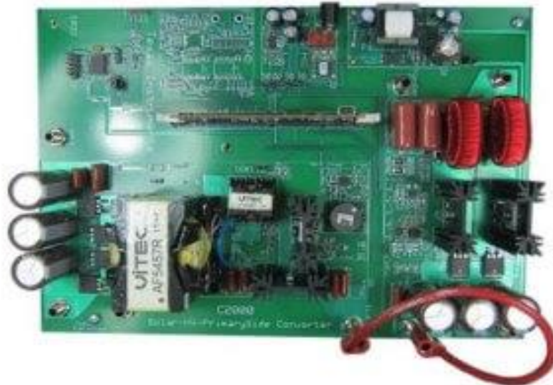
Figure 4.12.4a - DC to DC converter with MPPT. Reprinted with permission from Texas Instruments
