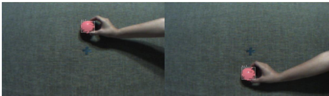
Figure 6.2b - Test Case 1 images. Captured in PixyMon. On the left, object moves up, Pixy Camera successfully tracks the motion of the object. On the right, object moves down, Pixy Camera successfully tracks the motion of the object.
