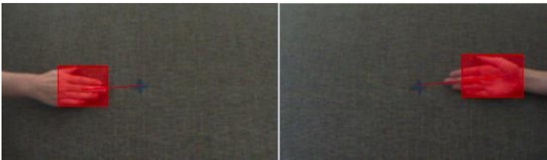
Figure 6.2g - Test Case 4 images. Captured in PixyMon. Red boxes show the region of motion being tracked by the Pixy Camera in relation to the center point of the frame.
