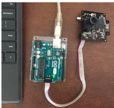
Figure 6.2f - Test Case 3 images. On the left, I2C connection between Pixy Cam and Arduino, Arduino connected to desktop via USB. On the right, image captured in Arduino serial monitor. Positional data being printed by the Arduino represents pixel coordinates of tracked object.
