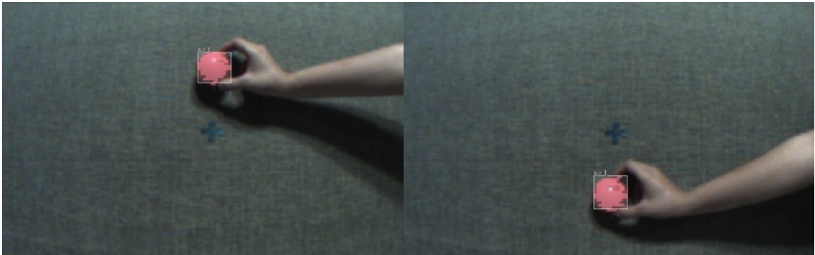
Figure 6.2b - Test Case 1 images. Captured in PixyMon. On the left, object moves up, Pixy Camera successfully tracks the motion of the object. On the right, object moves down, Pixy Camera successfully tracks the motion of the object.
