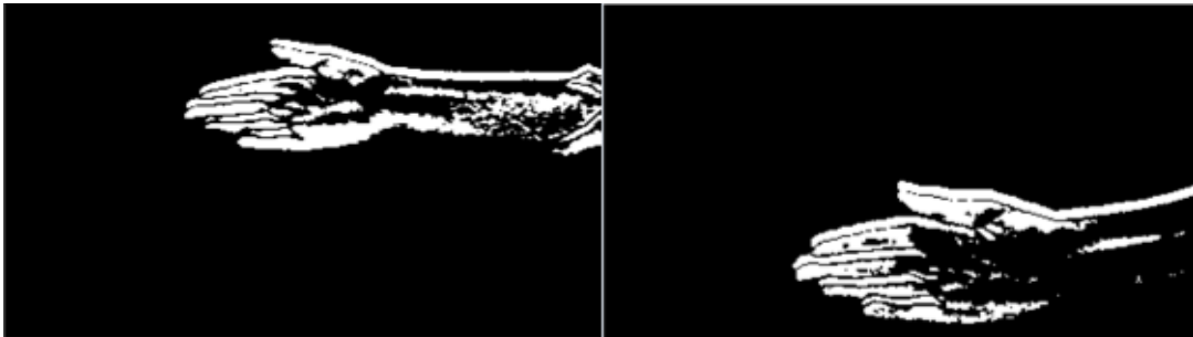
Figure 6.2g - Test Case 4 images. Captured in PixyMon. Image difference frames output by the Pixy Camera, motion is shown in white and static background is shown in black.
