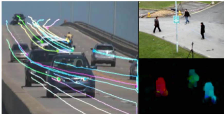
Figure 3.9.2a - comparison of sparse optical flow (left) with dense optical flow (right). Reprinted with permission from OpenCV Libraries
