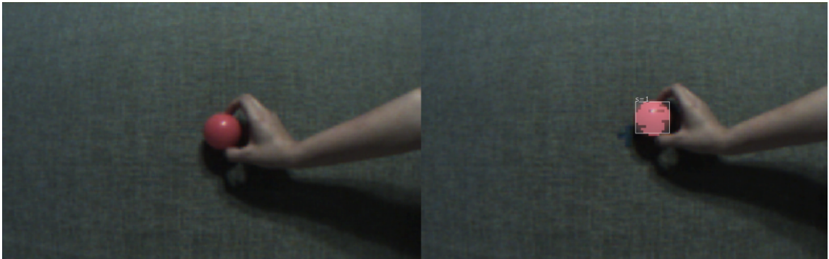
Figure 6.2a - Test Case 1 images. Captured in PixyMon. On the left, object to be tracked is presented to Pixy Camera. On the right, the Pixy Camera registers the object's color signature and begins tracking the object after being prompted by a command from PixyMon.
