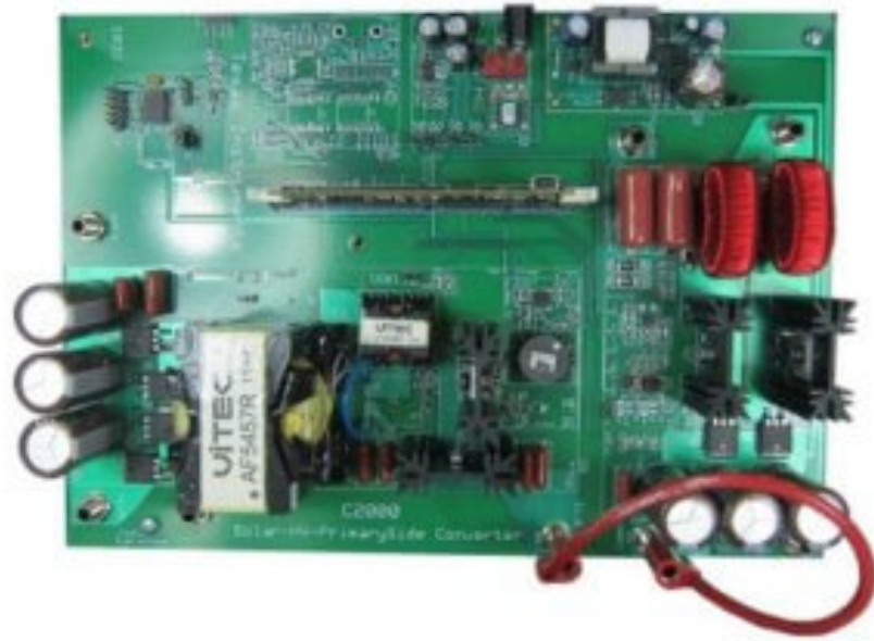
Figure 4.9.4a - DC to DC converter with MPPT. Reprinted with permission from Texas Instruments
