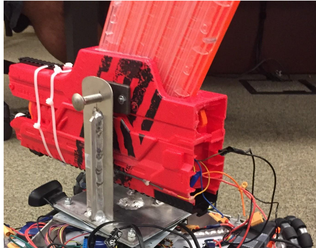
NERF Pan & Tilt system as designed by the M.E. team
