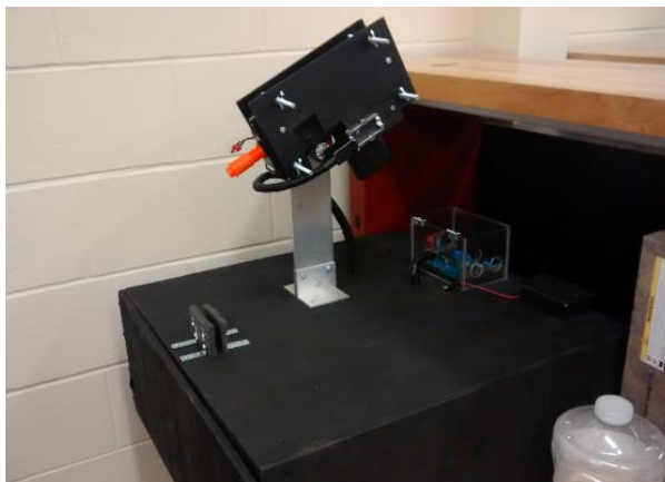
Figure 3.1.2 i: Self-Targeting Automated Turret System
