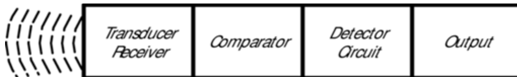
Figure 3.2.1.3 i: Ultrasonic Sensor Components Overview (approval pending)
