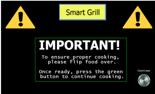
Fig. 6. Smart Grill LCD touchscreen prompts the user to flip the food being cooked to ensure proper cooking throughout.
