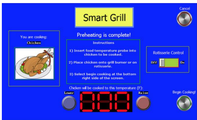
Fig. 4. Smart Grill LCD touchscreen displays the food prep screen for cooking chicken. User can set the desired cooking temperature, choose to use the rotisserie feature, begin cooking, or cancel and return to the main menu.
