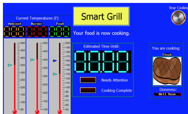
Fig. 5. Smart Grill LCD touchscreen displays the cooking screen for cooking steak. Temperature values are visible on the LED digits and thermometers. The estimated time until the meat needs to be turned over or is completed cooking is indicated in the center by the LED digits and virtual LEDs.
