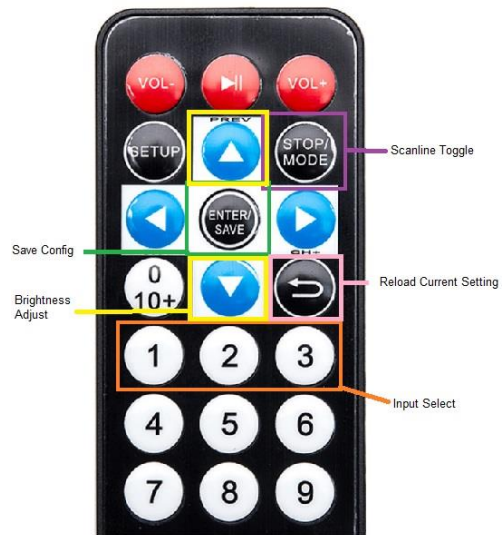
Fig. 8. The infrared remote control layout and supported settings in Super Doubler development.
