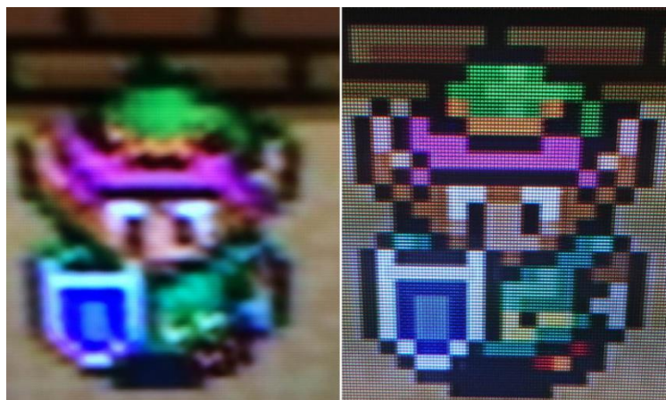
Figure 1: 240p signal. TV default processing mode (left), XRGB-mini device output (right).
