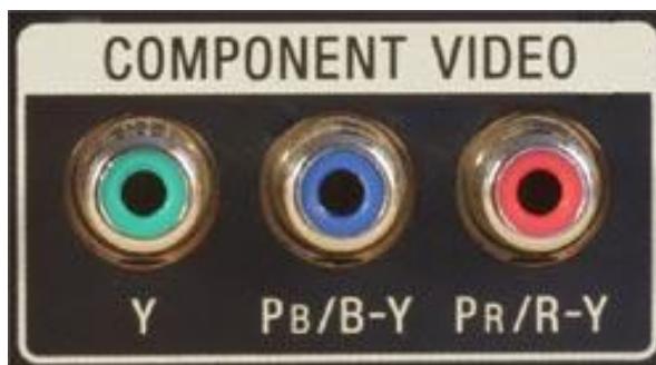
Figure 18: A set of RCA component video jacks. Courtesy of bluejeanscable.com.
