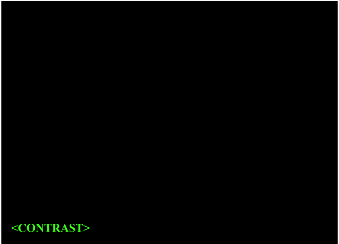
Figure 50. If the setting appears in green it means that the user is currently increasing the stored value of the setting.
