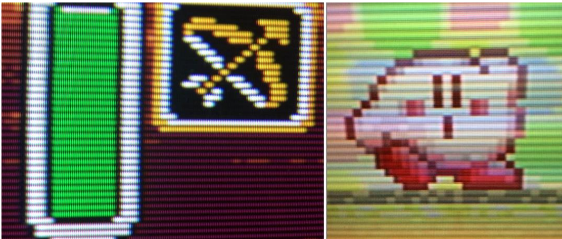
Figure 2: 240p signal displayed on a CRT television with darkened scanlines (left), emulated scanlines via XRGB-mini.
