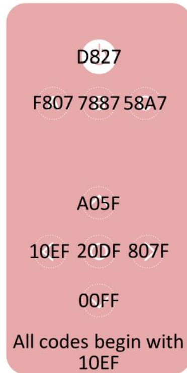
Figure 36: IR Remote Control with Input Codes. Courtesy of sparkfun.com.
