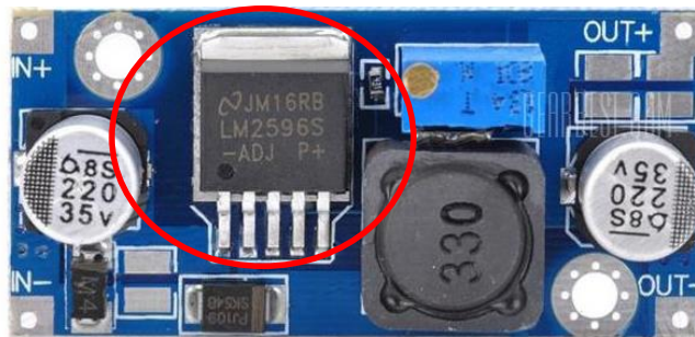
Figure 3.2.6 -1-: LM2596 Step Down Converter
