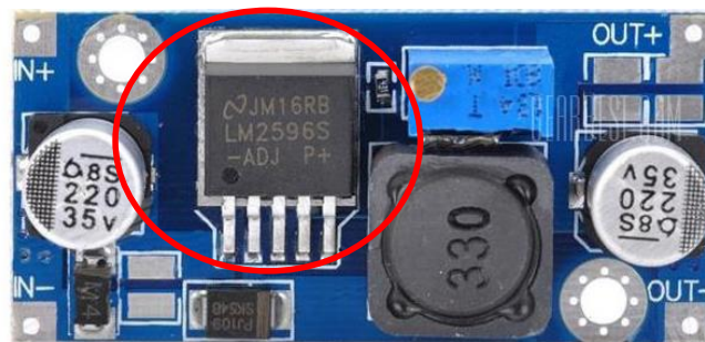
Figure 3.2.6 -1-: LM2596 Step Down Converter
