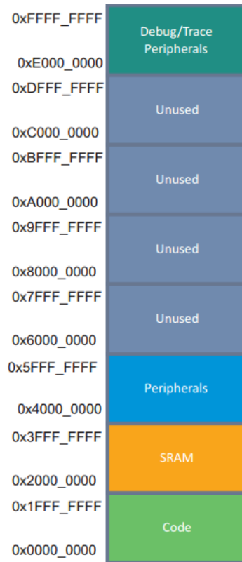
Figure 5.5.1.2-1: A general overview of the MSP432 memory layout Reprinted with the Permission of Texas Instruments
