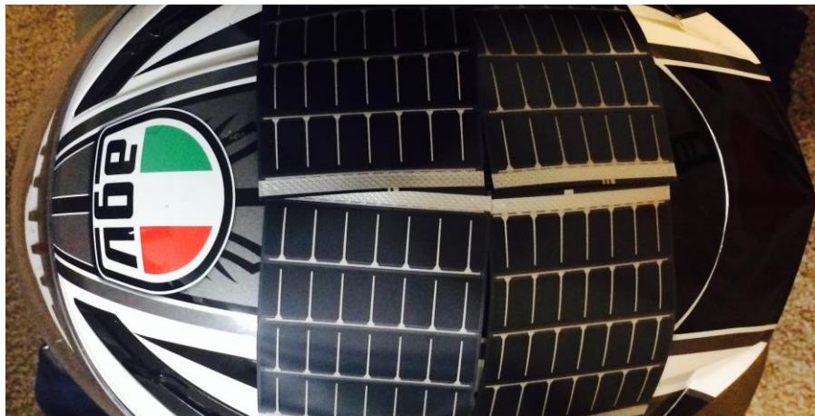
Figure 33: Solar Panel Placement Top View
