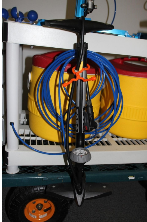
Figure 1-2: The bike pump is attached using a heavy duty twist tie. The students use it to pump air into the rocket through vinyl tubing (the blue tubing behind the pump). The pump has a pressure gage so the students can track the amount of pressure in the rocket.
