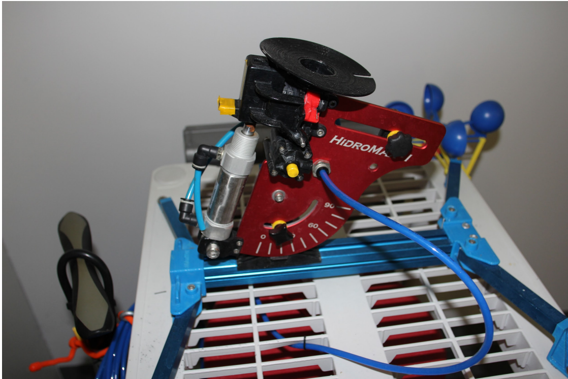
Figure 7-2: Close up of the launch pad for the water rockets. The nozzle of the bottle is inserted into the hole at the top of the black disk. Photo taken by SWR team.
