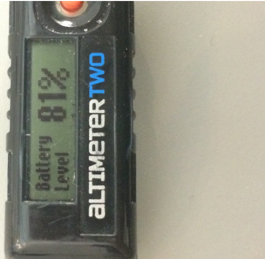
Figure 3-1: A photo of the AltimeterTwo used at Space Trek. The display (currently showing the battery level) is the only way to see data output from the device. Photo taken by the SWR team.
