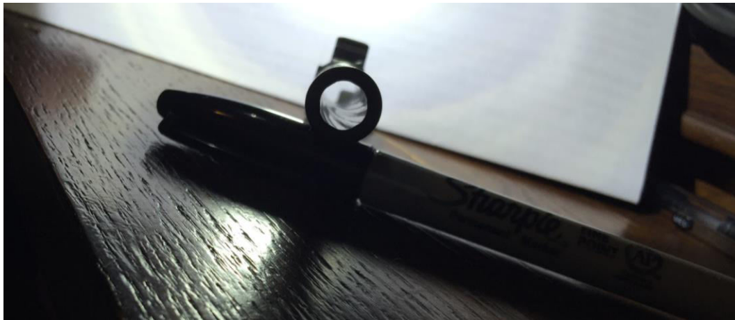
Figure 3.6: Rifling inside of Glock 18 Barrel
