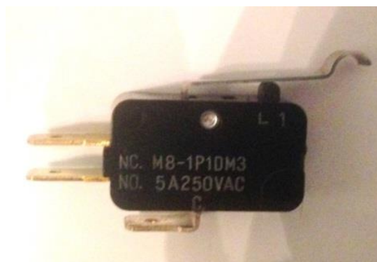
Figure 3.3.2-B Lift System Mechanical Micro switch Boundary Control
