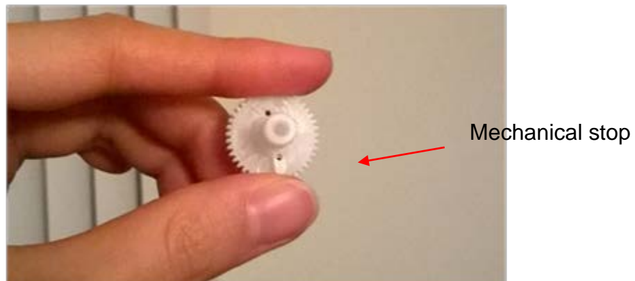
Figure 7-9: Top view of gear with mechanical stop
