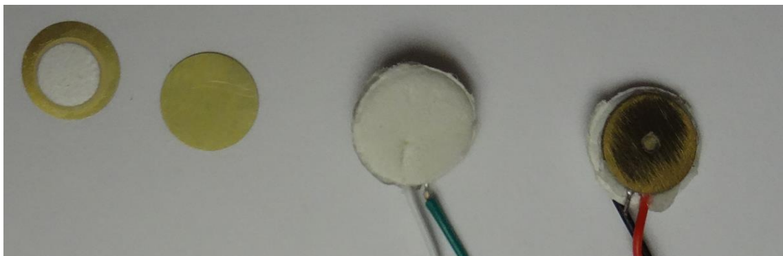
Figure 45: Bare piezo transducers (front and back) and finished sensors (front and back)
