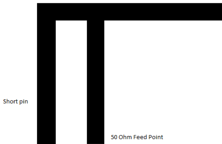
Figure 4.3.2-1 Above diagram shows a basic inverted-F antenna implementation.
