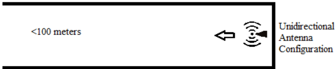
Figure 4.3.5-2 The above figure shown demonstrates the proper beacon placement of a unidirectional antenna in a long corridor
