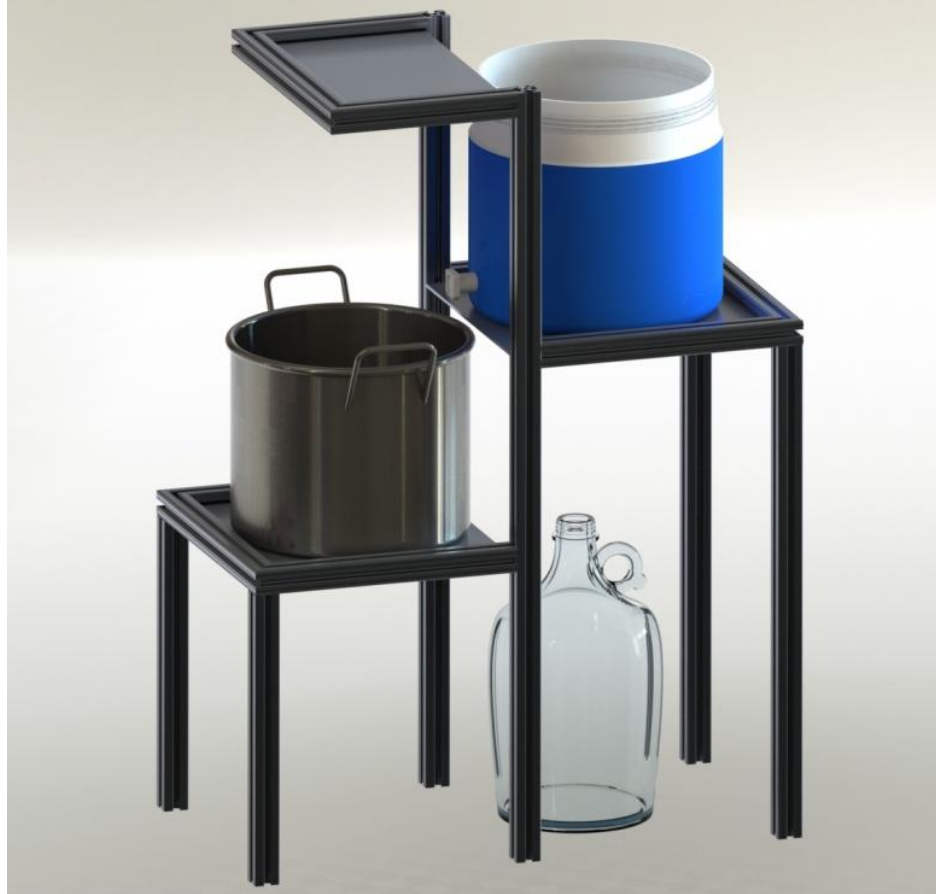
Figure 4.4: Configuration (b) using 80/20 extruded aluminum profiles.
