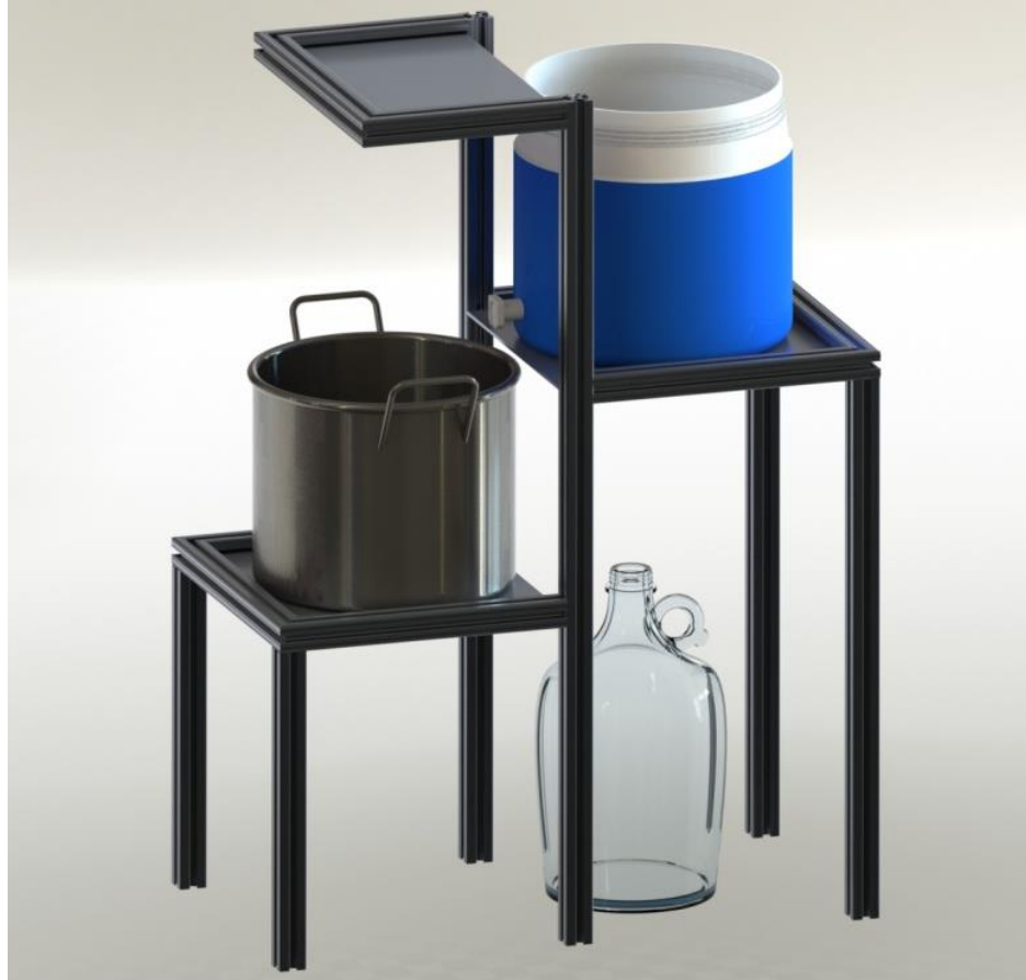
Figure 4.4: Configuration (b) using 80/20 extruded aluminum profiles.
