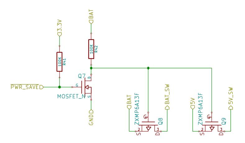
Power saving feature. All +5V and BAT subsystems are completely turned off.
