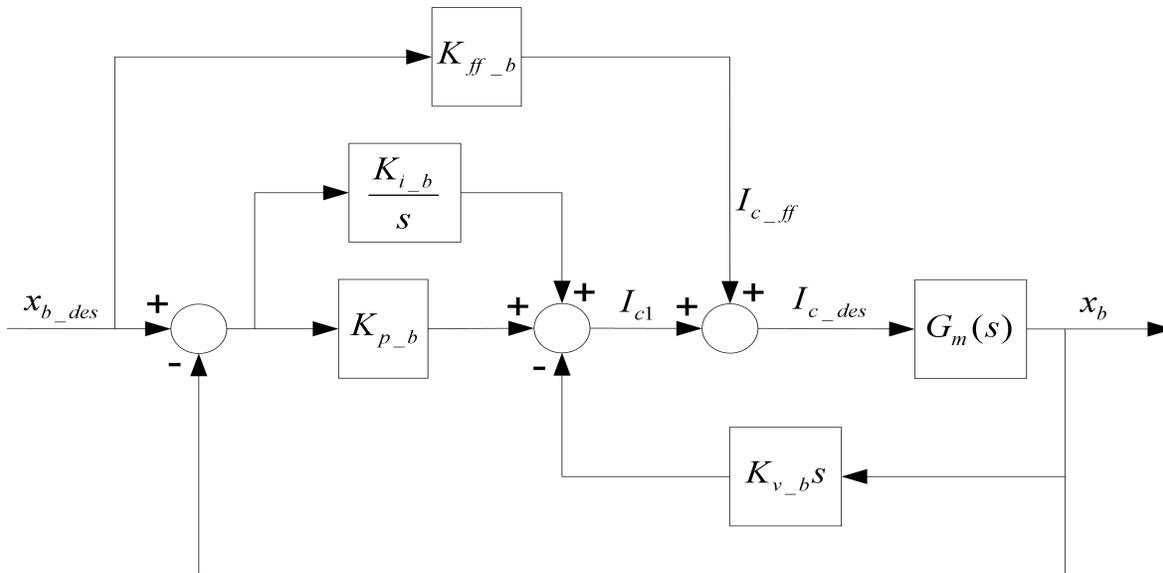
Figure 4 Ball Position PIV-plus-Feedforward Control Loop
