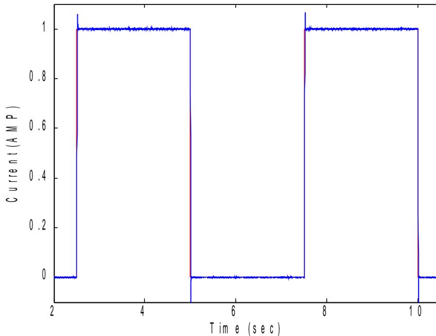
Figure 8 Actual  $I_c$  Response: PI Current Control Loop
