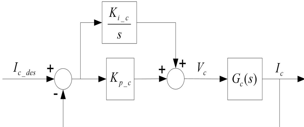
Figure 3 PI Current Control Loop
