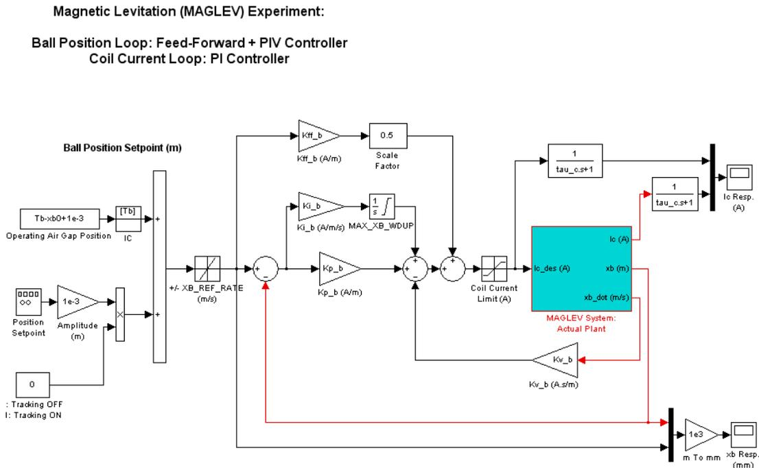
Figure 9 Diagram used for the Real-Time Implementation of the PIV Closed-Loop.
