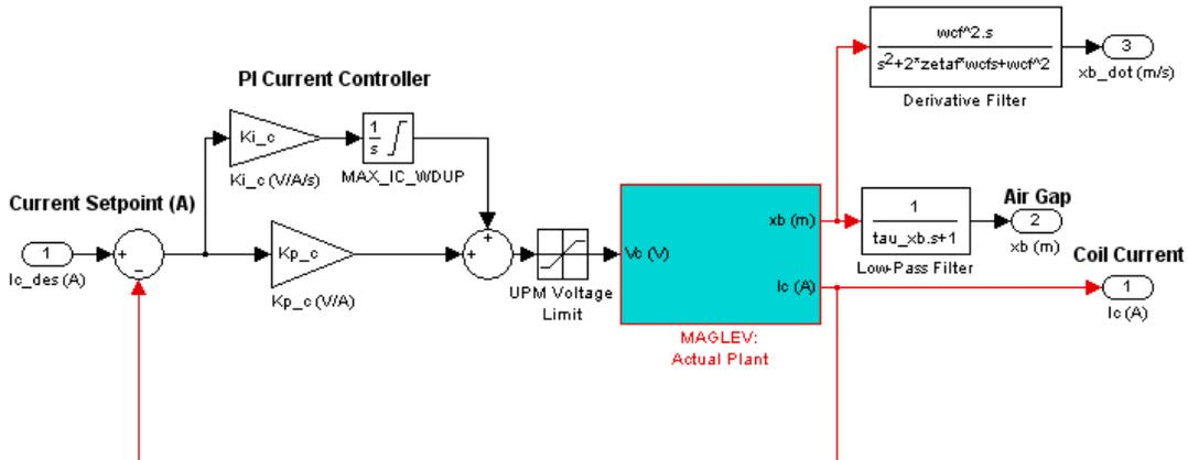
Figure 6 Real-Time Implementation of the PI Current Control Loop
