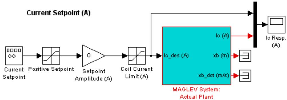
Figure 5 Real-Time Implementation of the PI Coil Current Control Loop And Setpoint Generation
