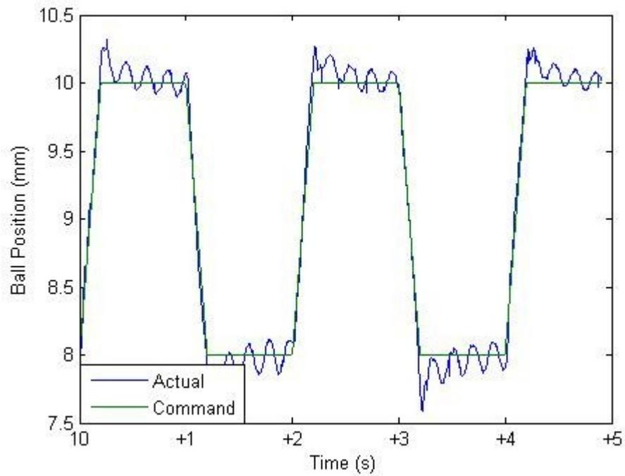
Figure 10 Actual Ball Position Tracking Response
