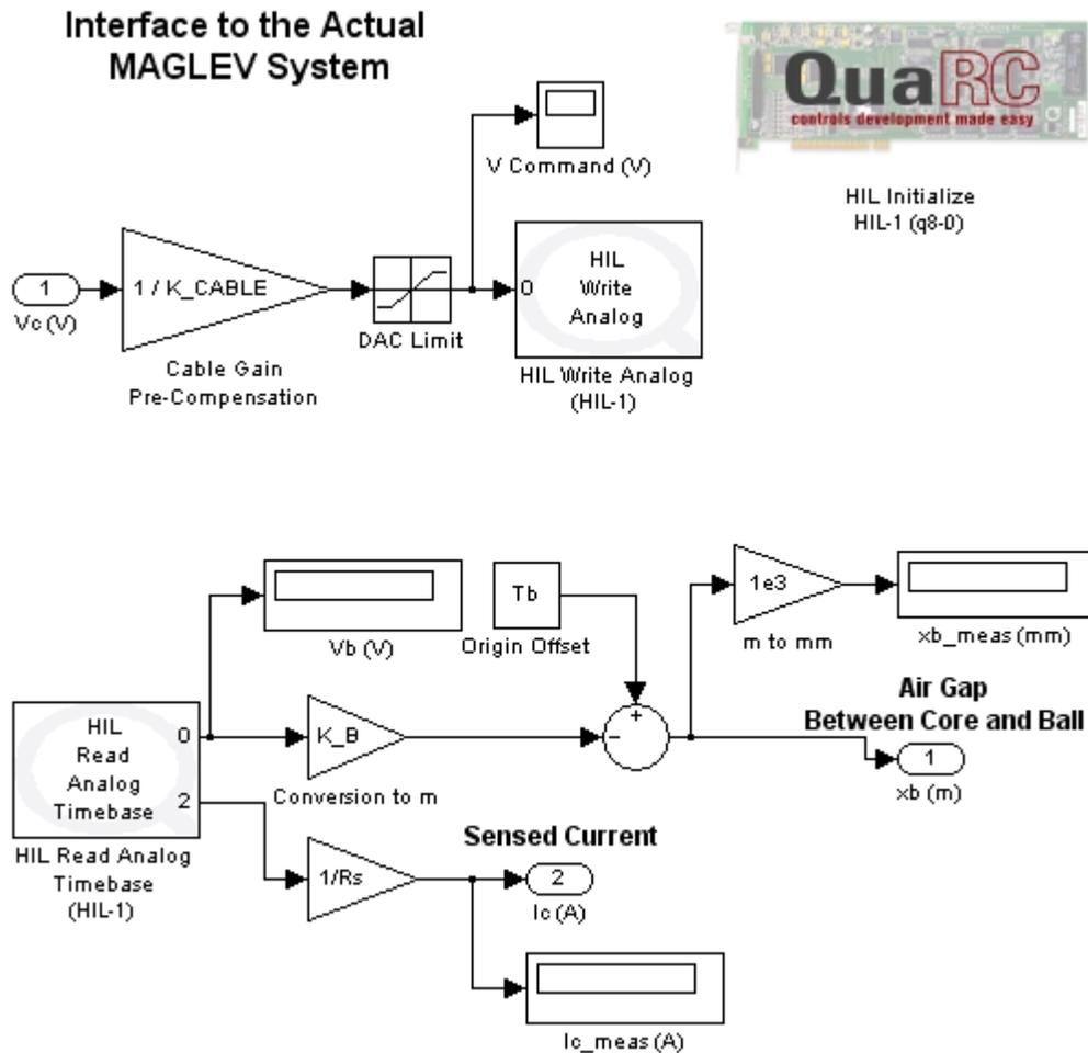
Figure 7 Interface Subsystem to the Actual MAGLEV Plant.
