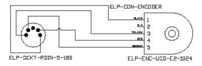
Figure 2.2: Encoder Wiring
