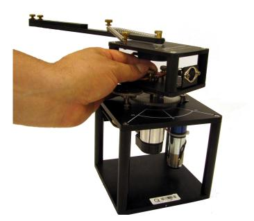
Figure 4.1: Attaching ROTFLEX to the SRV02
