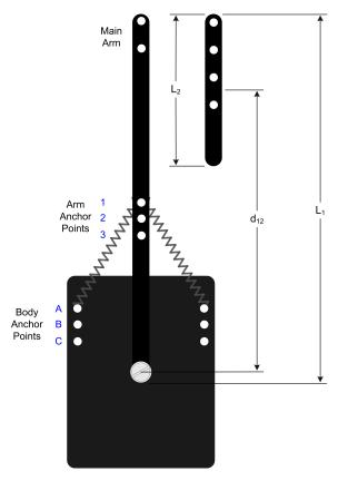
Figure 3.1: Rotary Flexible Joint Module
