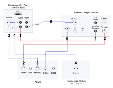
Figure 5.1: SRV02 and ROTFLEX Module Wiring Diagram
