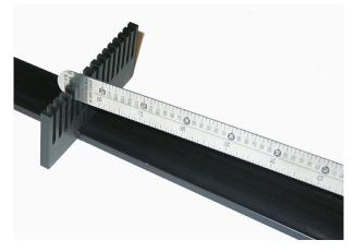
Figure 4.5: Flexible Link Tip Displaced by 1 inch in the Counter-clockwise Direction
