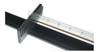
Figure 4.4: Flexible Link Tip Placed in the Middle Calibration Comb Slot
