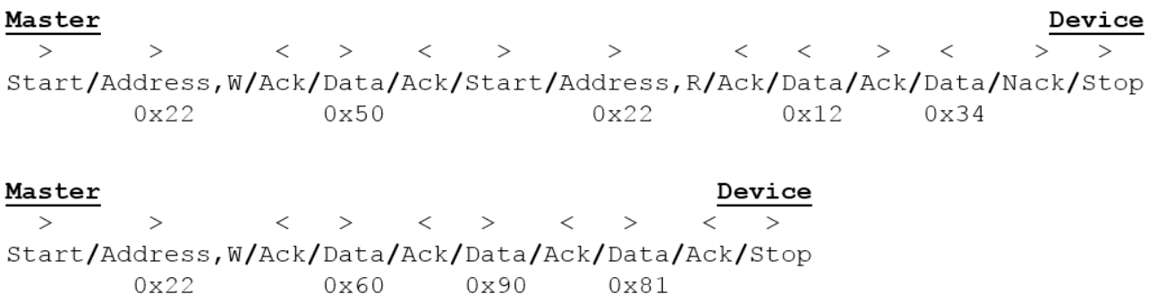
Figure 9.4: Read (top) and write (bottom) operations with the device's internal registers
