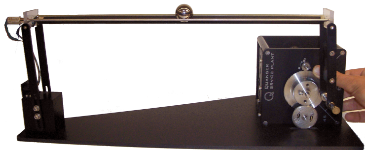
Figure 4.4: BB01 is calibrated when the centered ball is balanced on the beam while the SRV02 is at 0 degrees
